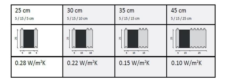
In the diagram above you can clearly see that the left part is the internal shell, right part the external shell. The black part is where the concrete and steel are coming.
