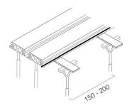
One of the most important and unique product properties is the continuous insulation, which is ensured partly by the connection with male / female profiles. The thickness of the floor slab can be kept to an absolute minimum and the U values can easily drop to  $0.17 \text{ W/m}^2 \text{ K}$ .
